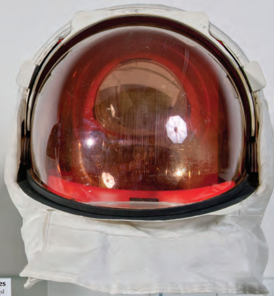
A7-L Lunar Extravehicular Visor Apollo 11 The visor assembly consists of a polycarbonate shell onto which the cover, visors, hinges, and eyeshades are attached. This helmet was worn over the suit's pressure helmet and fastened with a latch during Moon walks. It provided impact, micrometeoroid, thermal, and light protection. Transferred from NASA Johnson Space Center
